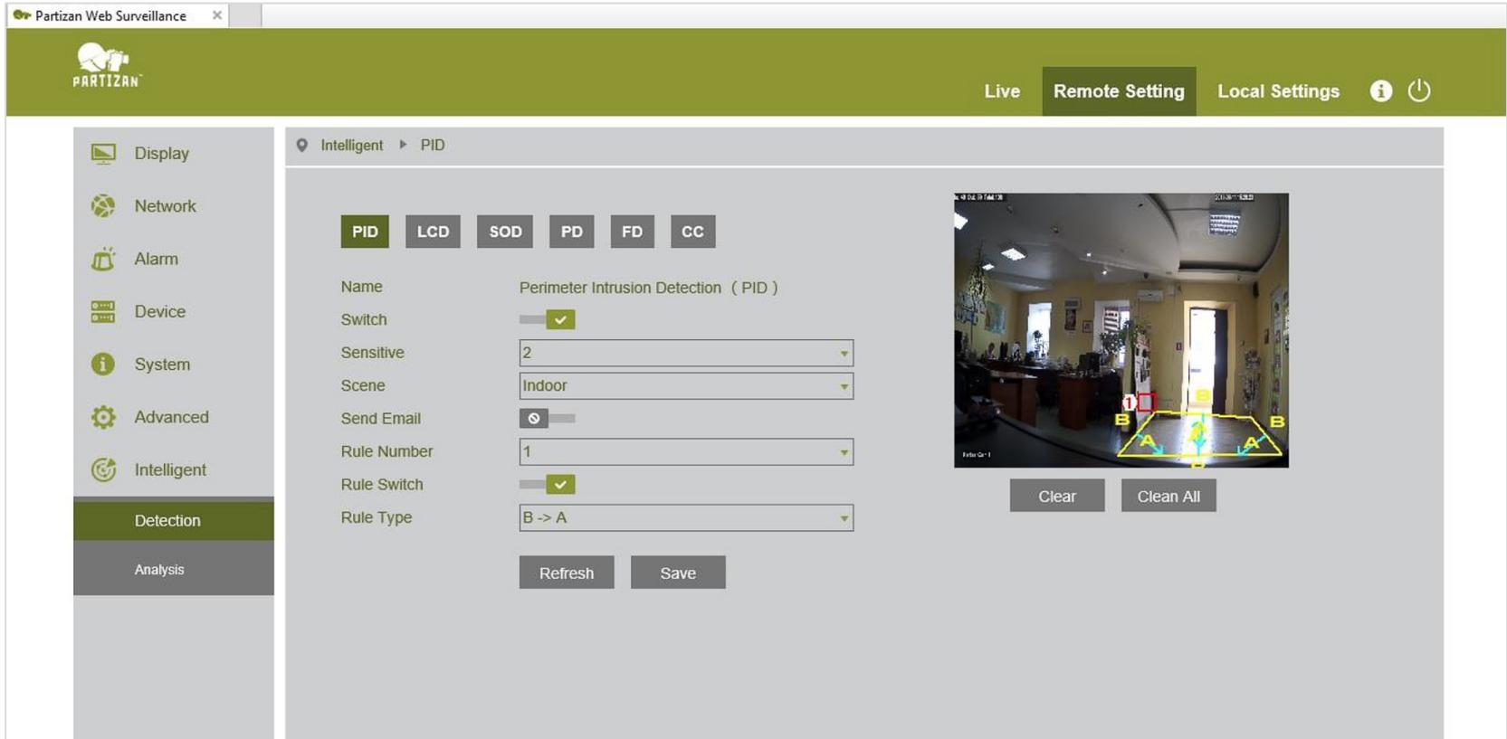
The screenshot displays the PARTIZAN Web Surveillance interface. The top navigation bar includes 'Live', 'Remote Setting', and 'Local Settings' tabs. The left sidebar contains a menu with options: Display, Network, Alarm, Device, System, Advanced, Intelligent, Detection (highlighted), and Analysis. The main content area is titled 'Intelligent > PID' and features several configuration options:
