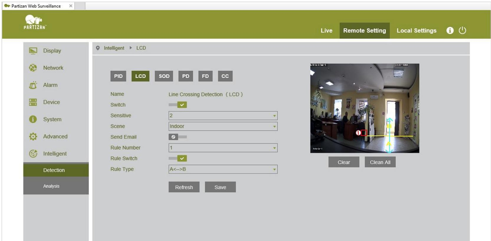
The screenshot displays the 'Partizan Web Surveillance' interface. The top navigation bar includes 'Live', 'Remote Setting', and 'Local Settings' tabs. The left sidebar contains a menu with 'Detection' selected. The main content area shows the 'Intelligent > LCD' settings page. The settings include:
